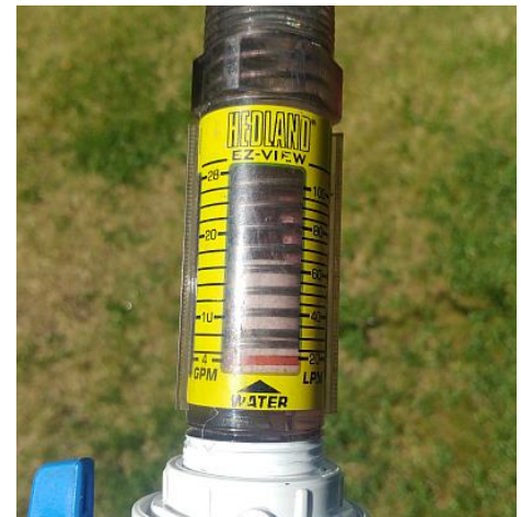
The flow rate is 6 gpm, which is within acceptable limits.
