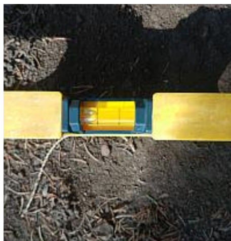
Negative grade observed in several areas. Recommend Repair (backfill).
