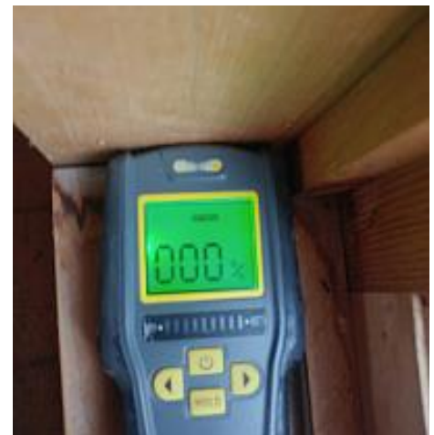
Moisture stains observed on the window sill. Although the area tested dry with a moisture meter, the stains came from somewhere. Recommend Repair.
