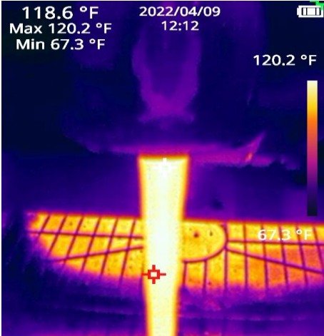
Water temperature is 120.2°F. A water temperature of 120°F is considered optimal for domestic use.
