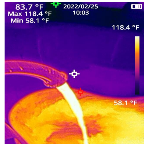
Water temperature is 118.4°F. A water temperature of 120°F is considered optimal for domestic use.
